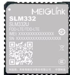
SLM332U is a new generation of LTE Cat1 wireless communication module, which adopts a domestic chip scheme, supports maximum downlink rate 10Mbps and maximum uplink rate 5Mbps; package adopts 17.7\*15.8\*2.4mm smaller size, convenient customer design size requirements, rich pin definition, meet the needs of customer multimedia and OPEN development.
